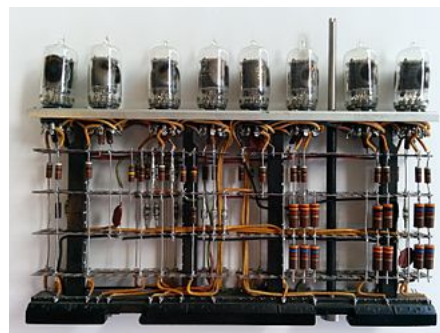
Vacuum tube logic module from a 700 series IBM computer.
